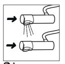
For the Pocket Tap Self-Priming (click valve tap). To activate the water flow, press the faucet from the front and hold. Release to stop the water
